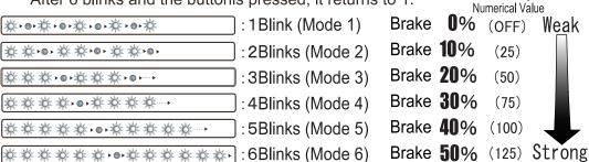
\*Factory default is mode 3. \*To finely set the 255 neutral brake phases requires using the ICS. To save the current setting, the power switch is turned OFF.
