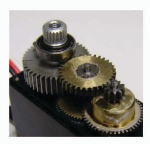
The grease that adheres to the gears originally is a white lithium based grease. If you have access to this type of grease, wipe off the old grease and re-grease all of the gears.
