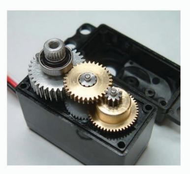
When the assembly or replacement of the upper case is done incorrectly, the original performance cannot be demonstrated with the use of the metal bushing in the upper case. This includes the KRS-2350RED servo. The explanation of the main points in the assembly are stated below.
