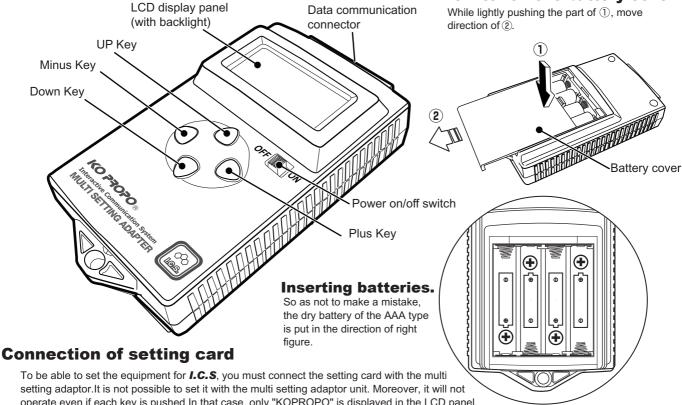
setting adaptor. It is not possible to set it with the multi setting adaptor unit. Moreover, it will not operate even if each key is pushed. In that case, only "KOPROPO" is displayed in the LCD panel.
