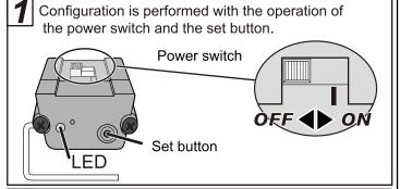
While pushing the set button, turn the power switch to ON. When LED lights up, the set button is released.
